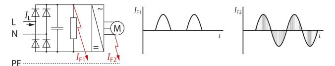
An insulation fault *IF1* on the DC side of the bridge rectifier produces a pulsed residual current at the fundamental (mains) frequency. This pulsed current may be superimposed on a smooth DC component, the effective value of which is related to the DC link voltage, smoothing capacitance, and fault resistance.
