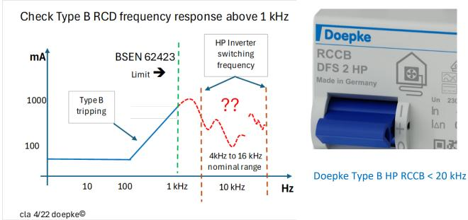
Refer to the manufacturer's Type B RCD technical characteristics, to verify their suitability for use with leakage currents generated by the HP inverter at frequencies > 1kHz. Doepke offer a range of tripping frequency response characteristics to suit domestic and industrial applications.
